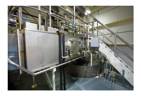
3,000 CFM of air is heated to >380 degrees F and enters the top of the dryer where it hits the product being atomized by the spray nozzle at >3,000 PSI.
