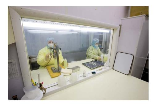
The bottling takes place in this Clean Room. The environment is controlled by supplying HEPA filtered quality air into the room. The radiation sterilized bottles are received into the plant in self contained modules and are not opened until they are ready to be filled.
