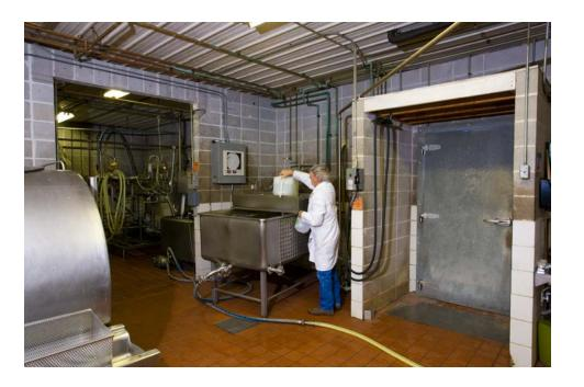
The curd is separated from the whey. The whey is then pasteurized, cooled and placed back in clean pails. The product is then refrozen; the product continues to be identified as to its source and processing stage.
