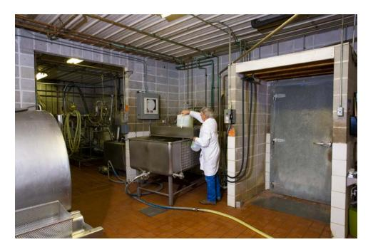
When a batch of product is scheduled for production. The appropriate formula sheet is consulted and pails removed from the freezer to meet the formula needs. The appropriate pails are removed from the freezer and the thawing process at room temperature begins. We complete the thawing process by transferring this product to a heat vat.
