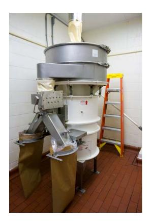
The powder is transported via pneumatic conveying lines into the receiver bag house and from there it is dumped into a sifter screen and then is placed in clean, clear plastic bags. The bags are sealed and placed in cardboard boxes and are staged for return to the Impro Plant.
