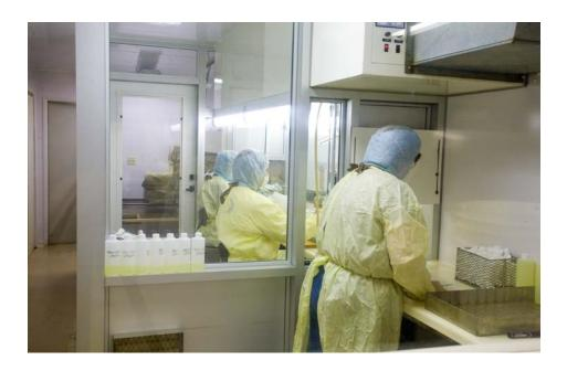
The whey is sterile filtered and the bottles are filled and stoppered under the HEPA filter.
